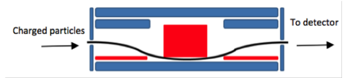
Figure 18: Schematic of the enhanced performance top-hat design for SWA-EAS under development for Solar Orbiter.
