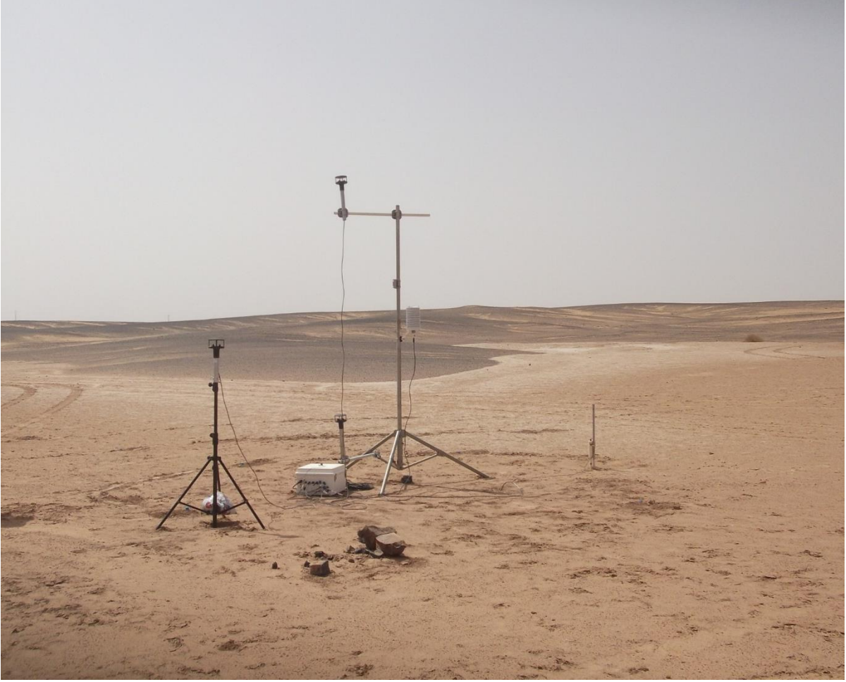
Fig. 1 The meteorological station deployed during the 2017 field campaign. The first small pebbles hill visible behind the station is located at \sim 30 m from it. The second line of higher hills is located at \sim 100 m.
