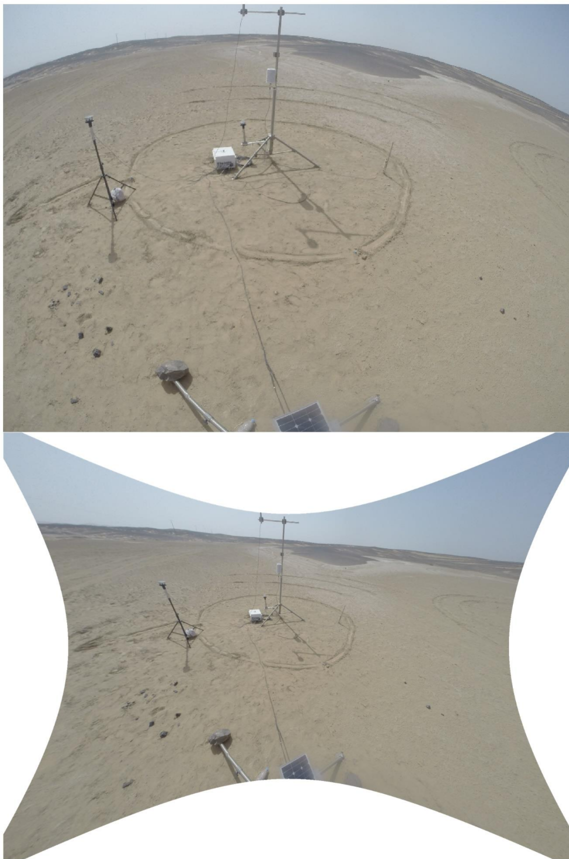
Fig. 3 One of the acquired images before (top) and after (bottom) the removal of the barrel distortion.
