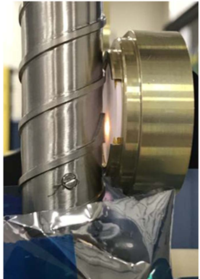
Figure 11. Ma_MISS lamp illuminating a spectral target during the measurements on the tip and rods in Leonardo Nerviano (MI).
