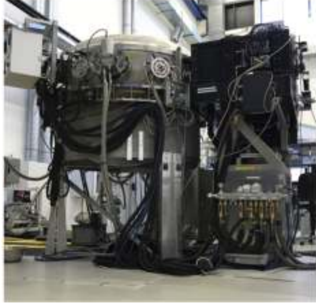
Fig. 8. Left: new CRIRES + warm part assembly with etalon system, calibration slide, AO system and de-rotator mechanism. Right: refurbished and enhanced warm part including the AO system mounted to the CRIRES + cold part during system testing at the ESO integration hall in Garching, Germany.
