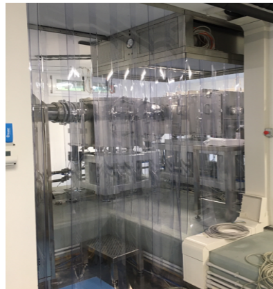
Figure 14. Left) the ISO5 clean tent. Right: the MM door opens into the clean environment
