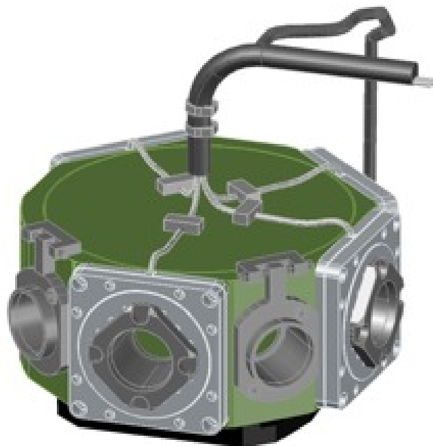
Figure 11. Mechanical design of the SPU. The turret carries beam-splitters and QWPs, some mounted on rotation stages. The whole turret can rotate around vertical axis.
