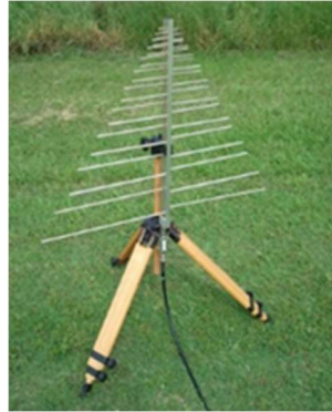
Fig. 8. The log-periodic antenna PMM LP-02
