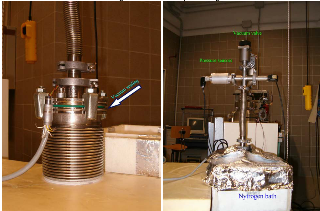
Fig. 1 The small chamber used in the tests(left) and a view of the vacuum setup (right). Also the pump is visible behind the Nitrogen bath.
