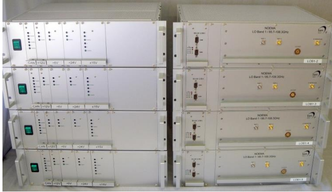
Fig. 13. The four production series of NOEMA Band 1 ( \sim 82 -108.2 GHz) LO racks (right) and their power supply racks (left).
