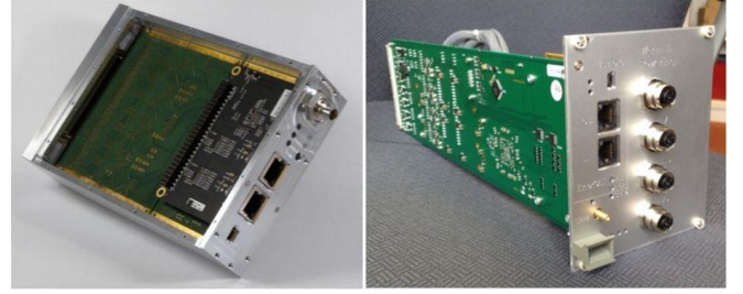
Fig. 18. EtherCat modules for biasing the NOEMA SIS junctions (left) and controlling the warm IF chain and laser rack emitter (right).
