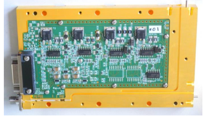
Fig. 11. Active Multiplier Chain developed for the NOEMA LO Band 1 system (AMC1) delivering a tunable signal across \sim 82 -108.3 GHz and a power level of order \sim 12 dBm at its WR10 waveguide output.
