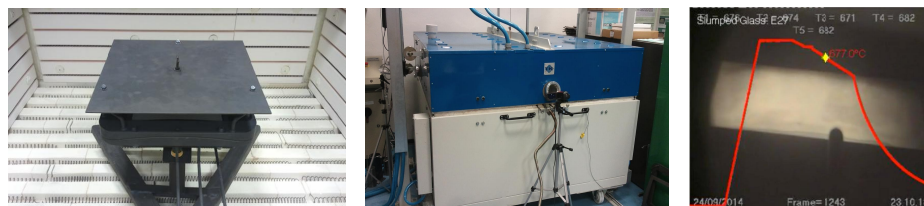
Fig. 2. Left: The muffle with the light open cover. Center: the furnace with the windows for the camera. Right: one shot of the movie of the change in the interference fringes, recorded during the slumping cycle.
