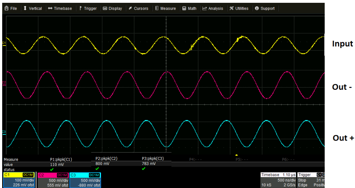
Figure 7. Preamplifier test with an external signal.
